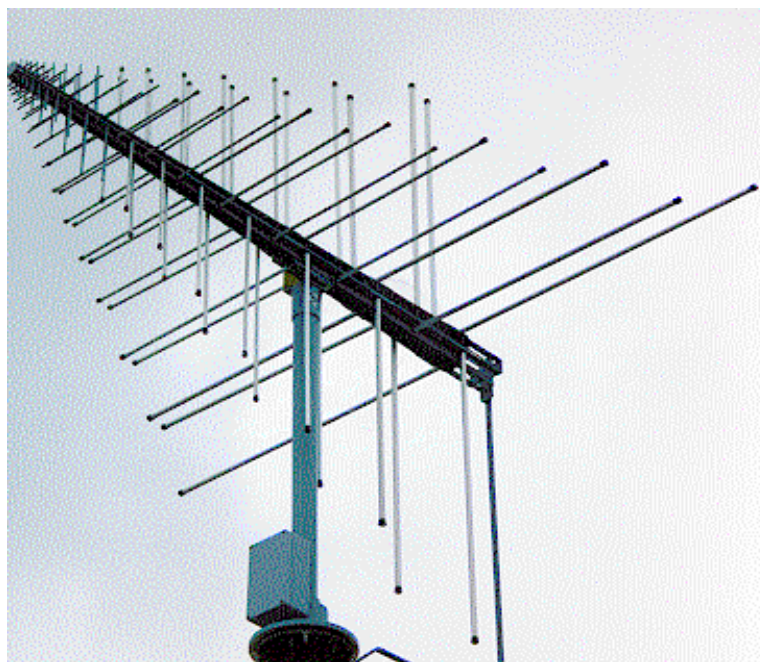
Fig. 4.32 Crossed log-periodic antenna for 80 MHz to 1300 MHz
