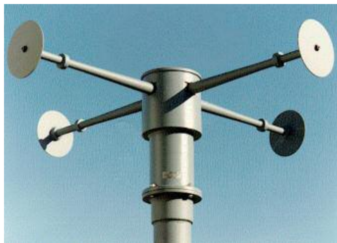
Fig. 4.17 Active turnstile antenna for 20 MHz to 500 MHz
