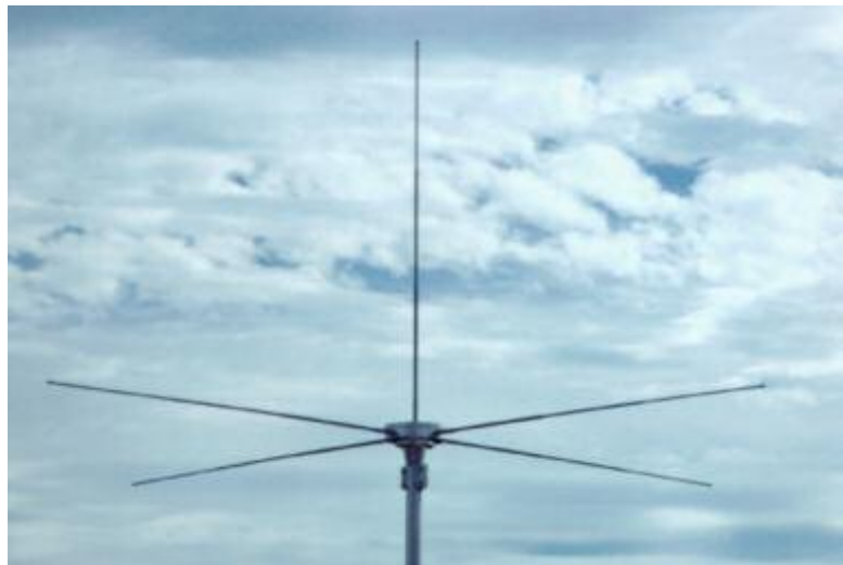
Fig. 4.19 Active turnstile antenna with monopole
